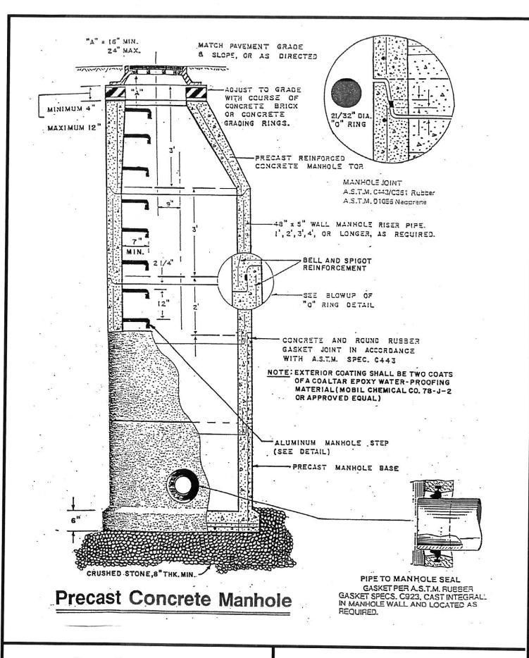
Precast Concrete Manhole Detail
